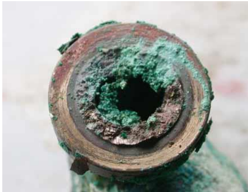
Figure 5.8 Copper pipe corrosion provided by Amtec Consultants
